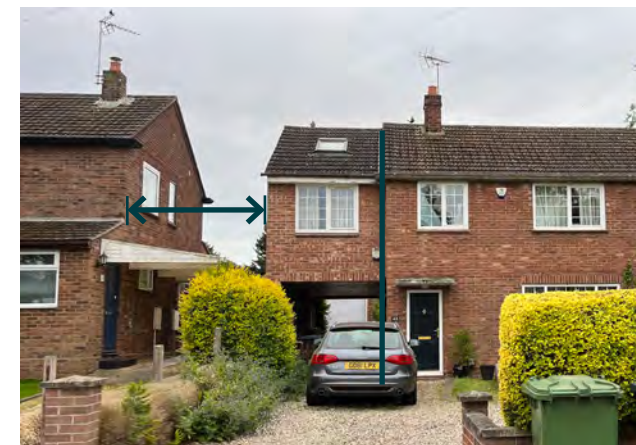
Figure 98: Outside example of a side extension with an inappropriate built gap, creating a terrace like streetscape.
