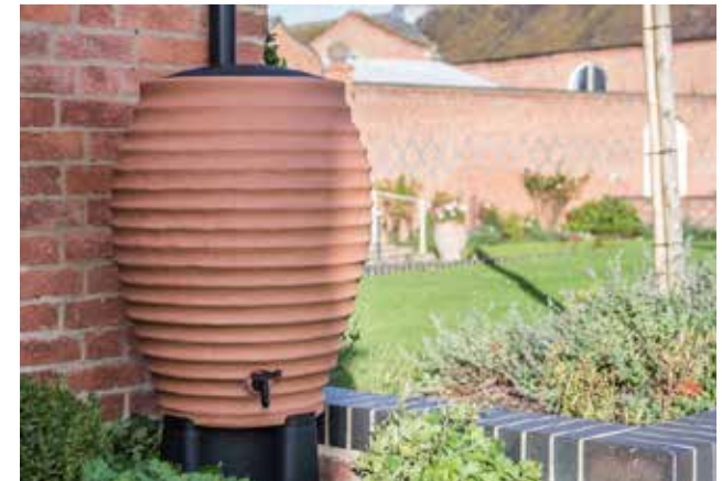
Figure 175: Example of a rainwater harvesting tank in the shape of a beehive (source: https://www.gardenplantsonline.co.uk/ )
