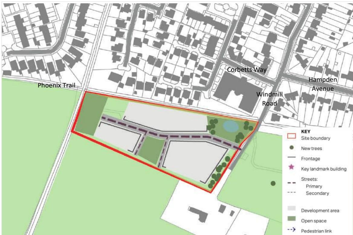
Figure 12: Concept masterplan for land at Windmill Road based upon design principles for the site. Further detail is set out in the *Thame Masterplanning Report*.
